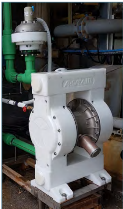
MISTRAL solid pump 3" for ceramic production plant (Italy)
