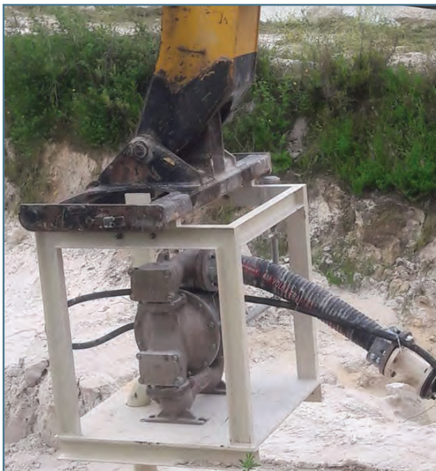
MISTRAL pump 4" for silice extraction (Italy)
